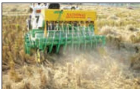
front of the tynes, places seed and fertiliser using zero till machine and push the chopped straw through the tynes on to the seeded area. This machine is capable of seeding into the loose residue load of up to 10 t/ha. This machine can cover an area of one acre per hour. It requires a tractor of more than 50 HP with a dual clutch.
